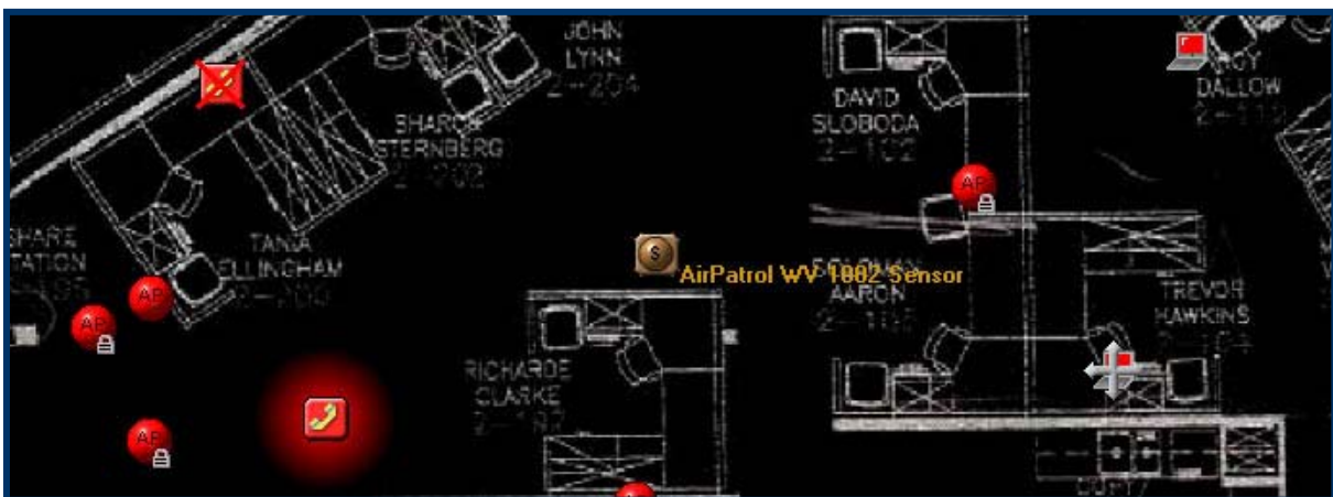
A detail from the Floor Plan console from AirPatrol's Wireless Locator System (WLS)
